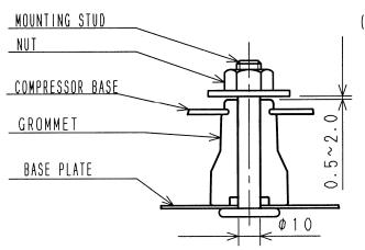
(THERE MUST BE CLEARANCE BETWEEN GROMMET & NUT.)
