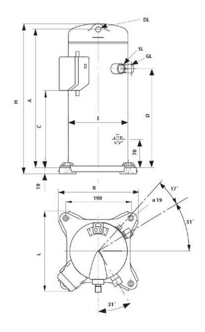
A B C D E H L 410 mm 240 mm 233 mm 297 mm 185 mm 457 mm 247 mm
